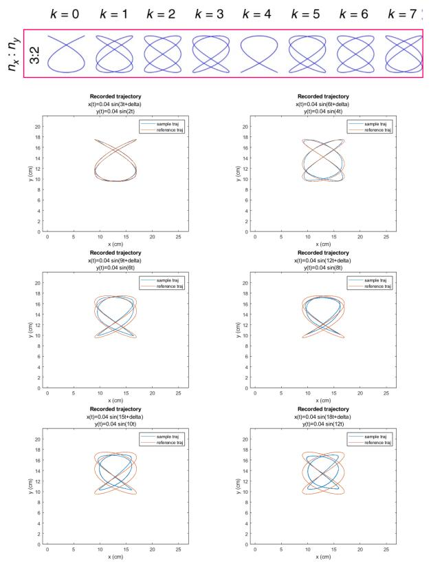
We can see that at  $\omega = 6$  rad/s (1st row, 2nd column) the distortion starts getting noticeable (controller+plant can't keep up with the desired trajectory).
